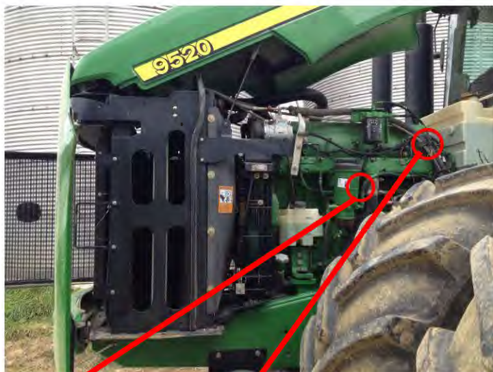
Fuel Pressure Sensor
